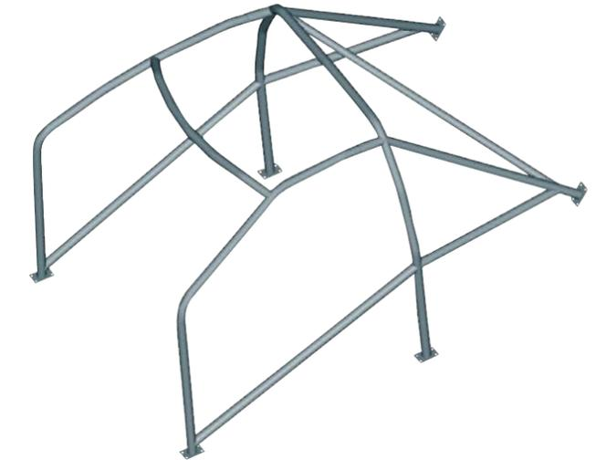
FE45 steel weld-in rollbars with Ø 50x2 tubing on the main hoop and Ø 40x2 tubing elsewhere. It may be necessary to remove or cut interior panels to facilitate installation.
