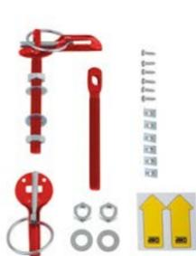
Quick release bonnet pins aluminium W 7/16" with stainless steel hardware.
