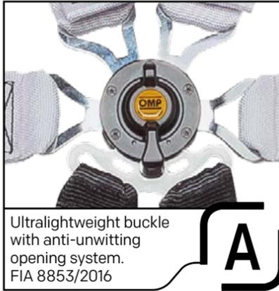
Ultralightweight buckle with anti-unwitting opening system. FIA 8853/2016
