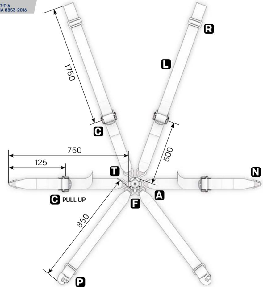
MEASUREMENTS IN MM
