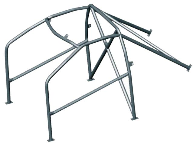
FE45 steel bolt-in rollbars with Ø 40x2 & 50x2 tubing, connecting sleeve tubes and reinforced brace in the main hoop. Supplied with door bars and diagonal reinforcement at rear.
