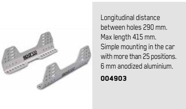
Longitudinal distance between holes 290 mm.
